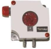
The PDE2-Series is designed to measure differential pressure in HVAC systems with non-flammable gases and non-aggressive gases. The control output is 2-point (ON/OFF). The differential switch has an internal set point adjuster.
