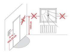
Mount the room thermostat on the cable conduit. Do not mount in niches or bookcases, behind curtains, above or near heat sources. Install at a height of about 1.5 meters from the floor. Devices must be mounted on clean, dry indoor place without direct airflow from a heating/cooling device. Do not expose to dripping or splashing.
