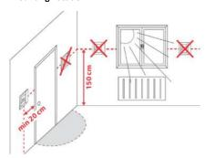
Mount the room thermostat on the cable conduit. Do not mount in niches or bookcases, behind curtains, above or near heat sources. Install at a height of about 1,5 meters from the floor. Devices must be mounted on a clean, dry indoor place without direct airflow from a heating/cooling device. Do not expose to dripping or splashing.
