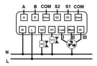
2-pipe: V1 Cooling/Heating valve
