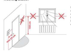
Mount the room thermostat on the cable conduit. Do not mount in niches or bookcases, behind curtains, above or near heat sources. Install at a height of about 1.5 meters from the floor. Devices must be mounted on a clean, dry indoor place without direct airflow from a heating/cooling device. Do not expose to dripping or splashing.
