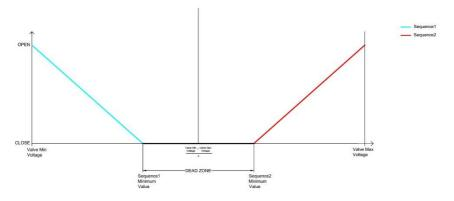
Sequence 1 is set as the default cooling valve. For Sequence 1 to operate in heating mode, it can be done by changing the Valve1 direction parameter.
