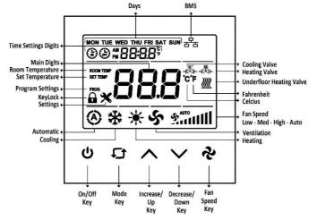
• Mode Selection: Press the MODE key to change the mode of the device. Active mode options are as follows.
