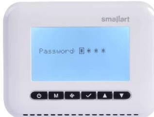
System Settings can be accessed by pressing and holding the **Menu** and **Down** keys together for 5 seconds on the main screen or by logging into the system settings menu from the user menu. The system setting menu can be accessed by entering the password “0203”. Switching between digits is made with the **Menu** key. The digit value can be increased or decreased with the **Up** and **Down** keys. The password is confirmed with the **Confirm** key.
