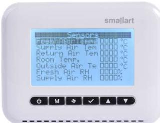
The Outside Air Temperature Sensor corresponds to the 1st bit. The Return Air Temperature Sensor corresponds to the 3rd bit. For these two sensors to be displayed on the sensors screen, set the "Active Sensor Buffer" parameter value to "4". For all sensor lines to appear, set the "Active Sensor Buffer" parameter value to "-1".
