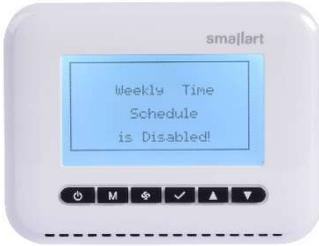
**Note:** If the "Weekly Time Schedule is Disabled!" warning is displayed after entering the weekly schedule screen, activate the weekly program enable point by making it "1".
