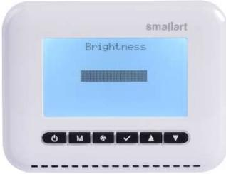
Screen brightness can be adjusted with the **Up** and **Down** keys.
