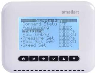
**ASP Screen Activation:** When Communication Parameter **182** is set to "1" the Aspirator screen opens.
