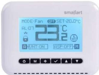
**Note:** When the Weekly Schedule setting is set to "Enable", the clock icon will appear on the screen and the on/off key will be locked. On/off control of the device will not be possible via the room panel.
