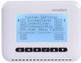
Technical user settings related to the panel are made in this section. To make changes in the parameters, select the parameter with the **Up** and **Down** keys. Select the parameter with the **Confirm** key. Change the digit value with the **Up** and **Down** keys. Switch between digits with the **Menu** key. Save changes with the **Confirm** key.
