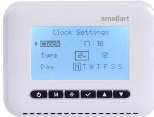
To open settings section, press **Confirm** key on the option that will change. Clock setting can be changed with **Up** and **Down** keys. Switch between hours and minutes with the **Menu** key. Changes made can be saved with the **Confirm** key.
