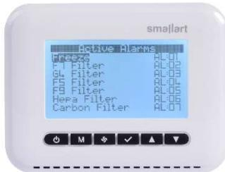
Freeze Alarm corresponds to the 1st bit. The F7 Filter Alarm corresponds to the 2nd bit. To display these two alarms on the alarms screen, set the "Remote Alarm 1" parameter value to "3". For all alarm lines to appear, set the "Remote Alarm" parameter value to "-1".
