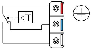
Heating: Connect to the red and blue terminal. The contact will open when the temperature rises..
