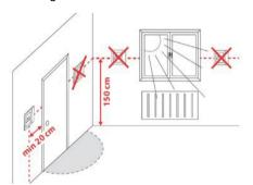
Mount the room thermostat on the cable conduit. Do not mount in niches or bookcases, behind curtains, above or near heat sources. Install at a height of about 1.5 meters from the floor. Devices must be mounted on clean, dry indoor place without direct airflow from a heating/cooling device. Do not expose to dripping or splashing.
